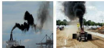
Incomplete Combustion: Excessive Black Smoke, Emission of Harmful Gases (COx, NOx)
