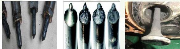
Incomplete Combustion: Excessive Black Smoke, Emission of Harmful Gases (COx, NOx)
